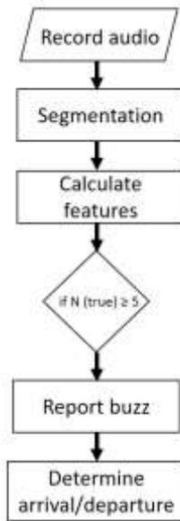
**Figure 1. Flowchart of the buzz detecting algorithm**
