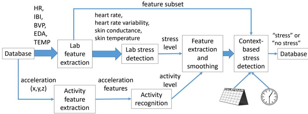
**Figure 1: An overview of the context-based stress detection model. Features are extracted from physiological signals from Empatica and input to a lab stress detector. Its predictions are used in the context-based stress detector, which in addition takes activity features from acceleration data into account and considers the time and the type of day.**
