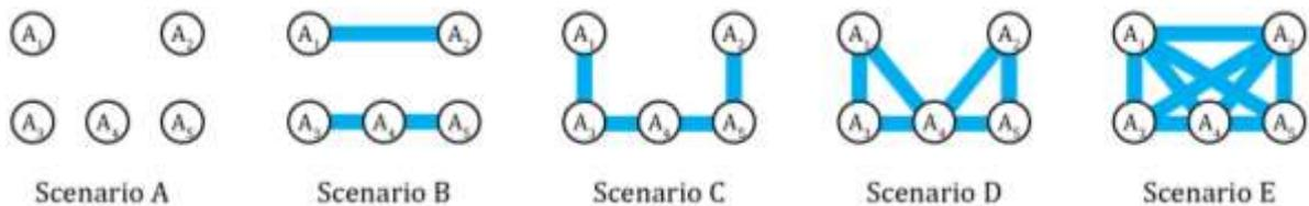
The total time of one simulation is set to 4000 s. Each scenario was simulated 150 times. The consumers' activity is random, each consumer is alternately set to on for 1 – 4 s and off for 30 – 40 s. The goal values of the compressor and the smart valves agents are set to 6.3 and 5.0 bar respectively and the safety valve has a set pressure of 10 bar for all scenarios.
